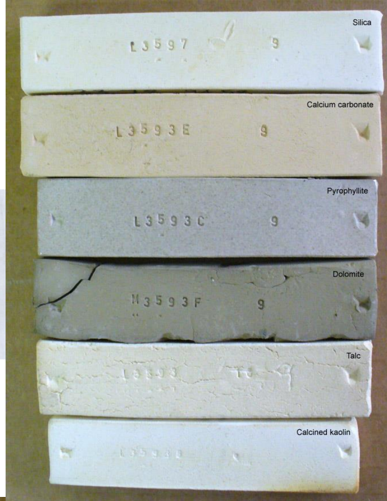
Examples of materials mixed with 25% vol clay bentonite and fired to cone 9
