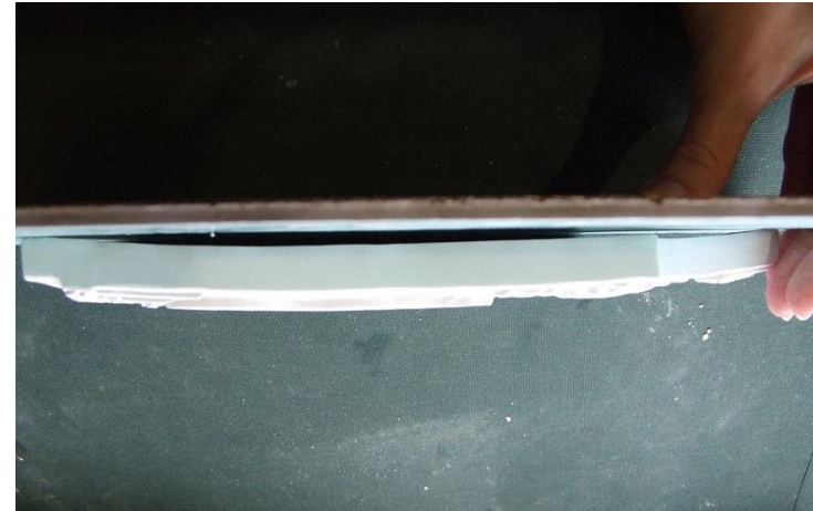
Fig. 24.6 Distortion produced by nonuniform drying shrinkage.
