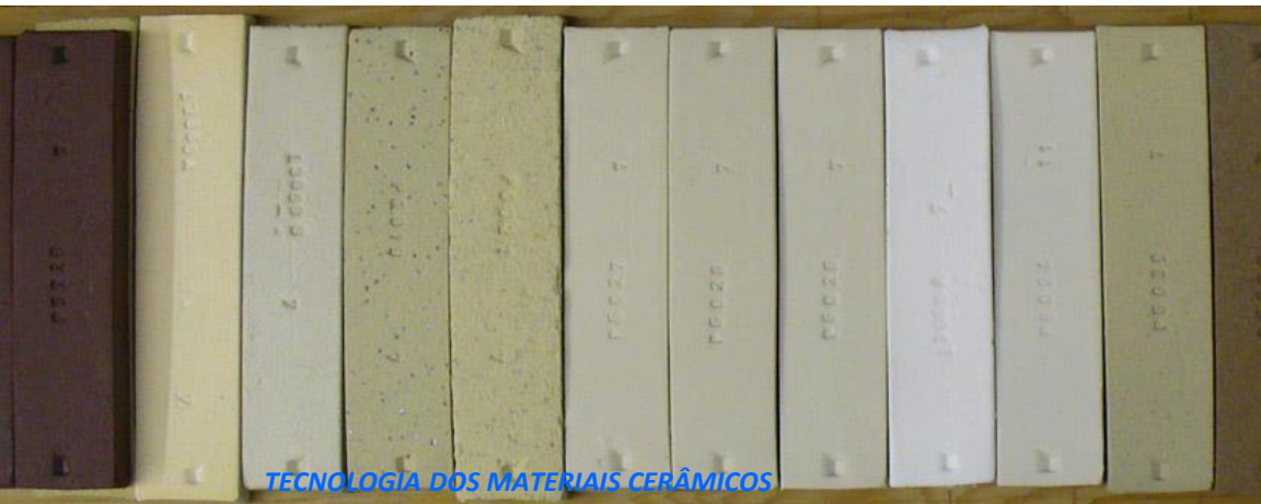
Examples of materials mixed with 25% vol clay bentonite and fired to cone 9
